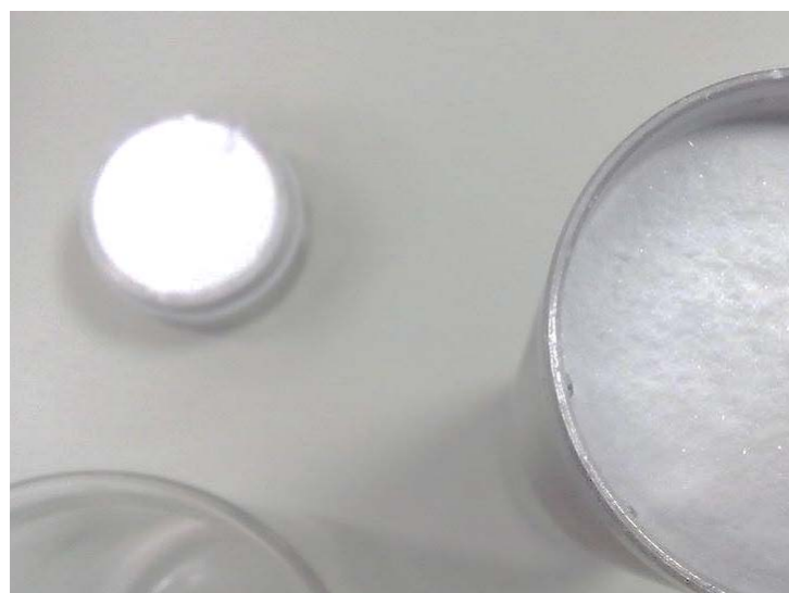
Image: Paracetamol powder after supercritical CO 2 extraction
