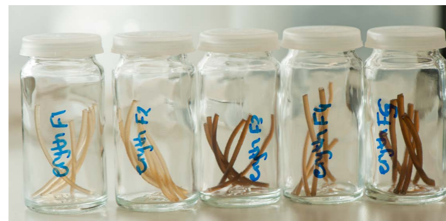
Image: Filament samples processed by HME
