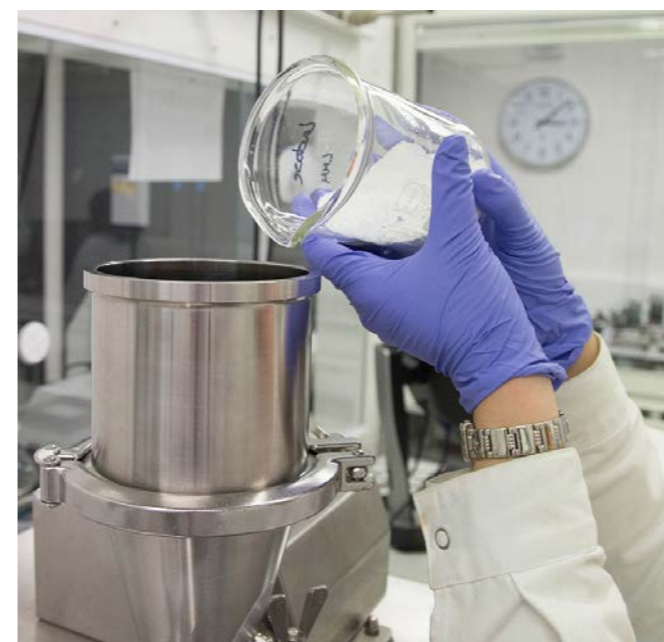
Image: Loading the twin screw granulator
