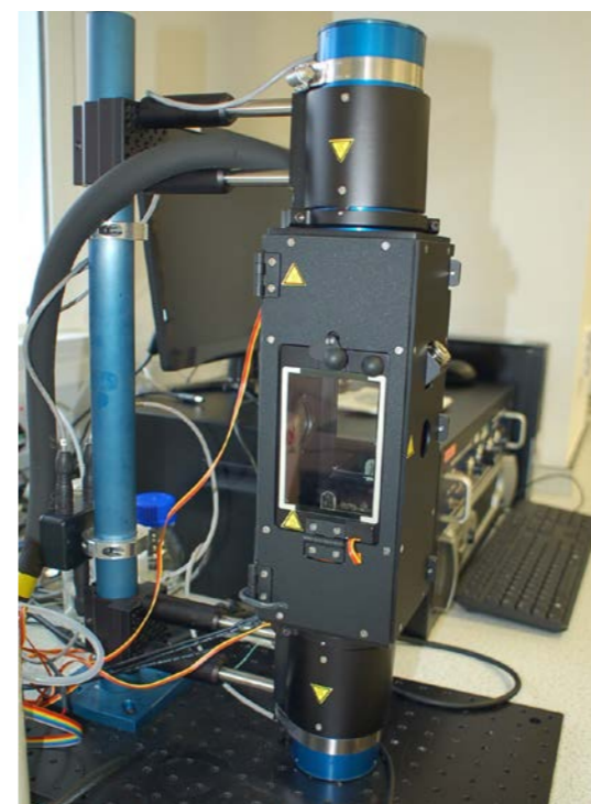
Single Droplet Evaporation Experiments (Acoustic Levitator)
