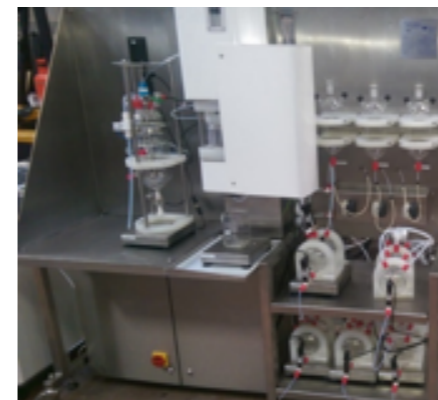
Image: Strand 1: Continuous drug substance filtration: AWL lab scale prototype
