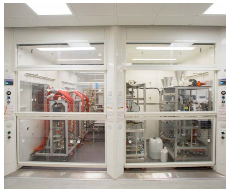
Image: Custom made reconfigurable integrated modular crystallisation miniplant housed in CMAC National Facility
