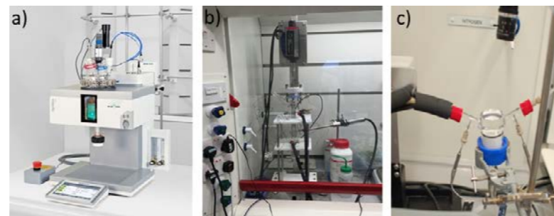
Figure 17. Examples of platforms used in Stage 5 a) Optimax, b) MB-OBC and c) fouling cell.
