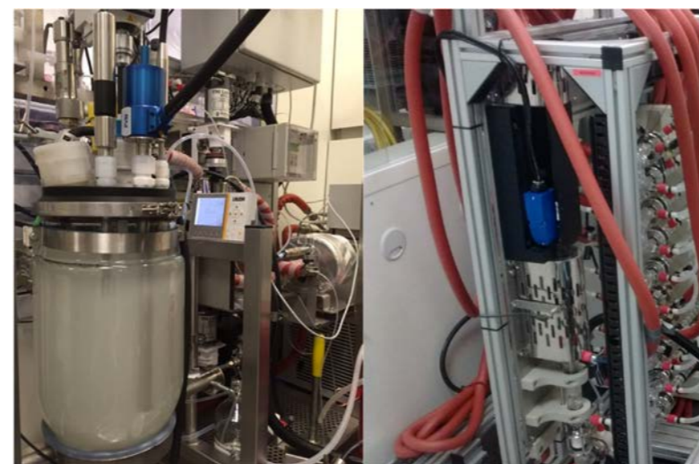
Figure 19. Modular skid mounted crystallisers utilised in Stage 7.
