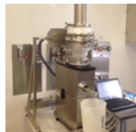
Image: Strand 2: Continuous direct compression: GEA CDC50 test rig, PAT enabled, for continuous feeding, blending and compression
