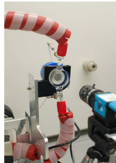
Figure 45. Image of the developed flow cell comprising an optical window for monitoring of the investigated MOC and incorporation of Pt100 sensors to monitor the efficiency of heat transfer
