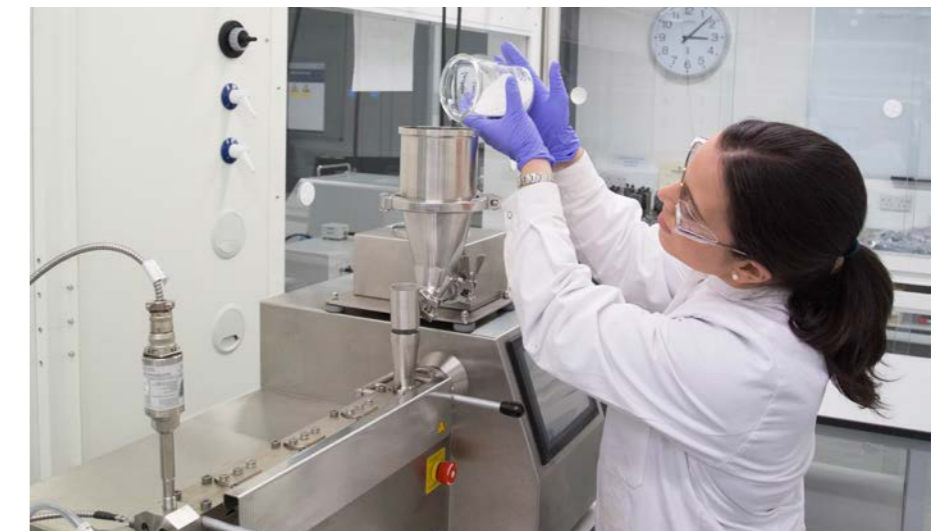
Image: Feeding API into the Twin Screw Granulator
