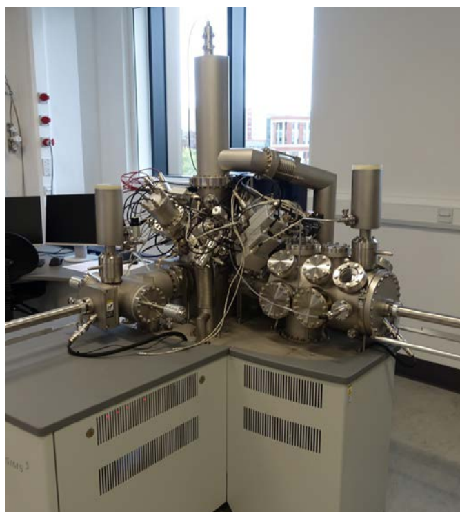
Image. TOF-SIMS Instrument in CMAC National Facility
