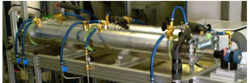
CRD's Rattlesnake Continuous Crystalliser
