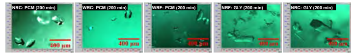
Figure 4. PVM images of product crystals obtained after 200 minutes periodic flow crystallisation experiment with GLY and PCM. NRC/F = No recycle and coarse /fine seed; and WRC/F = With recycle and coarse /fine seed.
