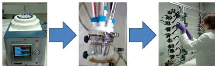
Scale-up of urea-barbituric acid crystallisation from small scale cooling crystallisation in the PolarBear (Cambridge Reactor Design) through to continuous crystallisation using the COBC.
