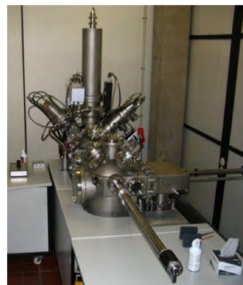
Figure 1. An indication of the complexity of a TOF-SIMS instrument. This instrument will be housed in a dedicated facility on Level 6 in TIC.
