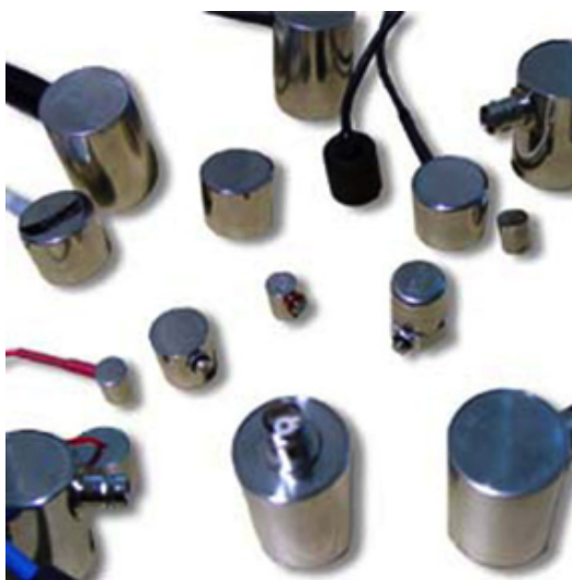
Figure 19. Physical Acoustics Site transducers
