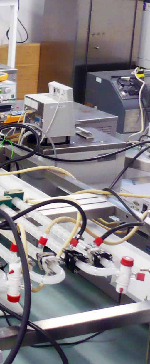
Figure 5. Nucleator Set-up for antisolvent crystallisation of \beta LGA seed crystals
