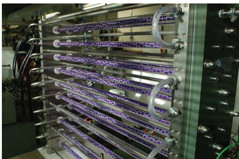
Figure 14. Continuous oscillatory baffled reactor (above) and AFM image of crystal growth on crystal surface (right).
